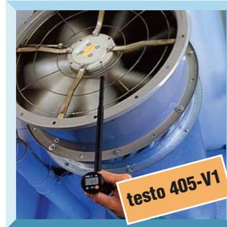
**testo 405-V1** is the first mini anemometer in this price range which can measure air velocity **and** volume flow.
