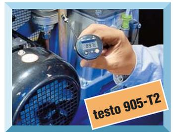
**testo 905-T2** The sprung, wide thermocouple measuring head, type K, guarantees a very quick reaction time and a high accuracy level by placing the probe flat on the uneven surface.
