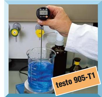
**testo 905-T1** is ideal for super-quick measured results in liquids, air and in soft or powdery substances.
