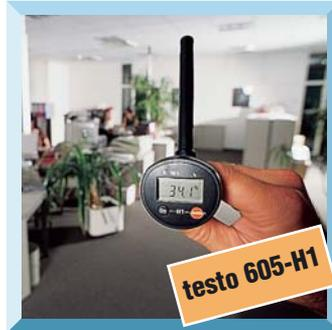
**testo 605-H1** The humidity measurement stick with the trick. Small, compact and accurate. It can be attached to your breast pocket via the push-on clip.
