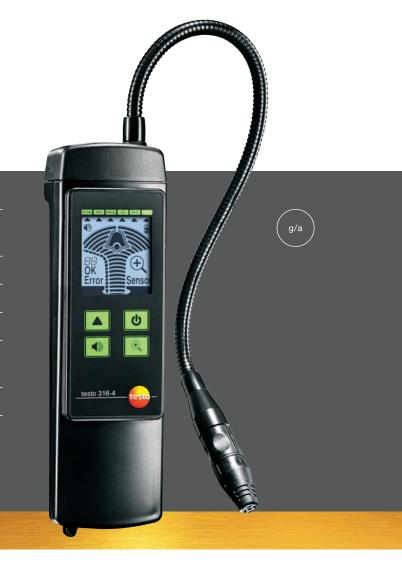
The testo 316-4 (Set 1) is a fast and reliable leakage detector for all common refrigerants. The sensor is permanently monitored and shows malfunctions or contamination in the display. The use of test leaks is thus superfluous. If dirty, the sensor can simply be cleaned, and is immediately ready for use again.
