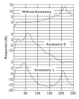
Frequency(Hz) HI range 8. Contact resonance in acceleration measurement: (worked with FFT signal analyzer)
