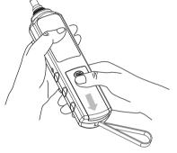
b. Insert the 9V battery into battery compartment, note the battery polarity, and then close the battery door, as shown in following figure:
