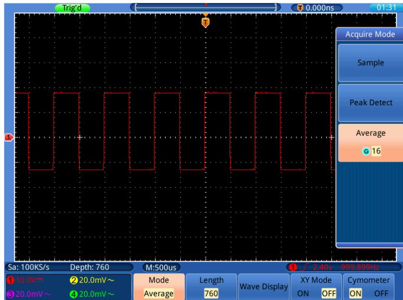
Figure 7-5 Reduce Noise level by using Average function
