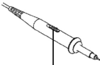
Figure 4-8 Attenuation Switch
