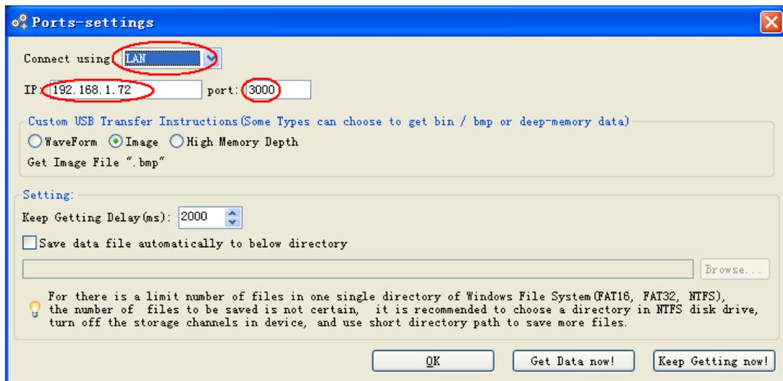
Figure 6-3 Set the network parameters of the Software
