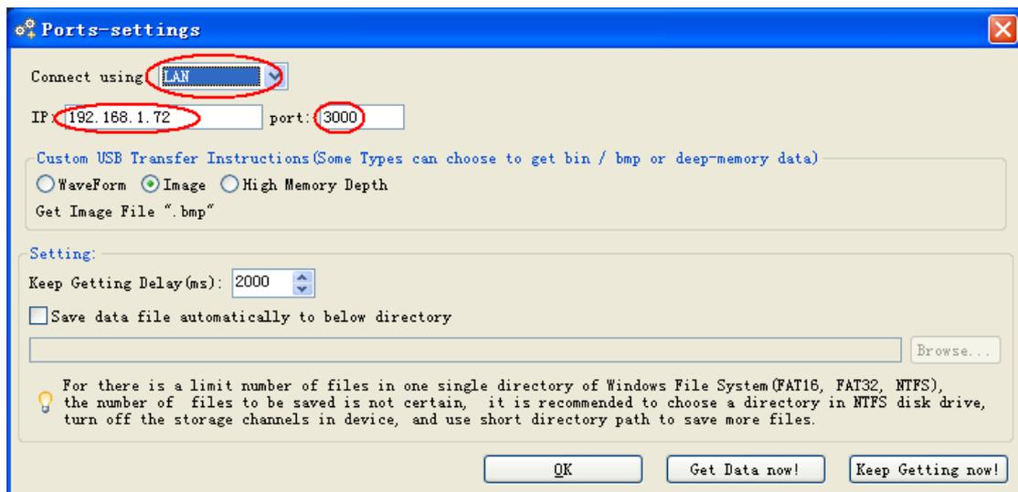
Figure 6-6 Set the network parameters of the Software
