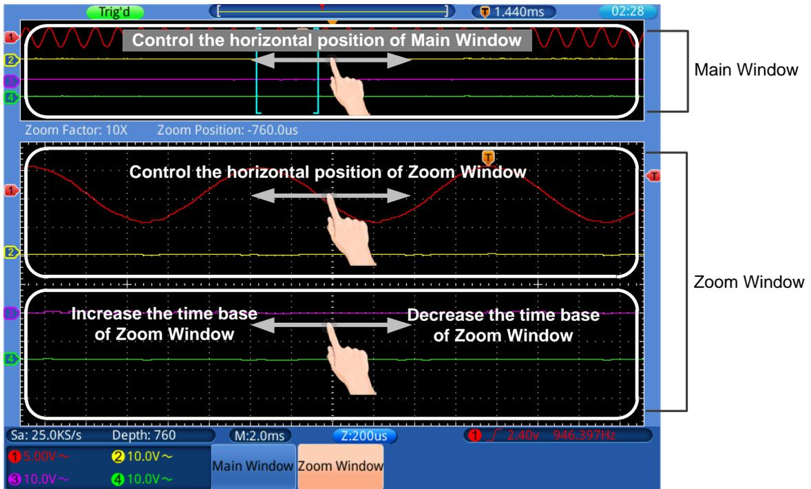
When **Main Window** in the bottom menu is selected, the horizontal operations using touchscreen are shown in the figure below:
