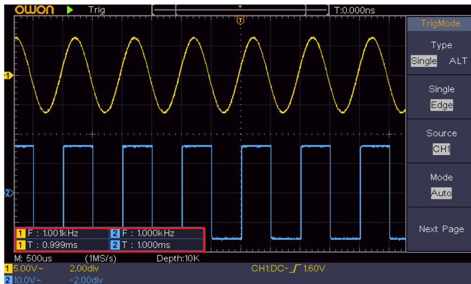
Figure 4-12 Automatic measurement
