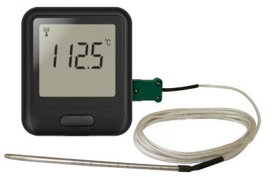
During configuration, the sensor will search for an existing wireless network whilst physically connected to the PC. It can then be placed anywhere within range of the network. If the sensor temporarily loses connectivity with the network, it will log readings until it is able to communicate again with the PC application or FilesThruTheAir<sup>™</sup> Cloud (max 30 days at 10 second sample interval).
