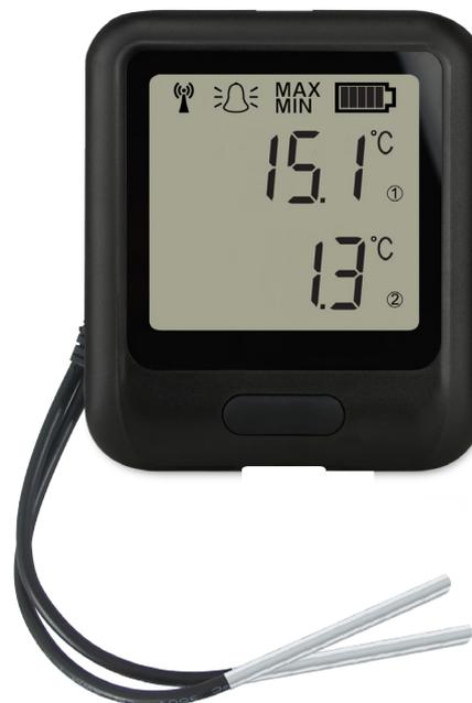
The EL-WiFi-DTP+ datalogging sensor measures the temperature of the environment in which the two probes are situated. This high accuracy sensor is typically accurate to  $\pm 0.2^{\circ}\text{C} / \pm 0.4^{\circ}\text{F}$  (+15° to +80°C/ -5° to +176°F). The unit is freestanding, but can be attached to a wall or surface using the bracket provided. The unit can be clipped in and out of the bracket as required. The probes are connected to the sensor via a 160mm Y splitter cable which is provided.
