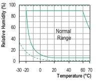
Long term exposure to humidity levels outside of the 'normal' range may temporarily offset RH measurements ( $\pm$ 3%RH after 60 hours). Once returned to less extreme conditions the device will slowly return towards calibration state.
