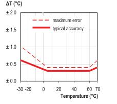
SENSOR ACCURACY & INFORMATION Typical and maximal tolerance for temperature sensor in °C.
