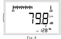
For 1/1 octave frequency, the center frequency changes according to  $31.5hz \rightarrow 63Hz \rightarrow 125Hz \rightarrow 250Hz \rightarrow 500Hz \rightarrow 1.0khz \rightarrow 2.0khz \rightarrow 4.0khz \rightarrow$
