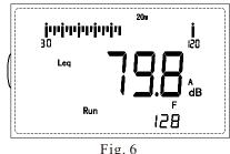
The Leq and integration time are displayed. At this time, checked whether the measurement time of equivalent continuous sound level meets the requirements. Confirm that it is correct. Then press the **RUN/PAUSE** key to start the equivalent continuous sound level measurement according to the preset requirements. The RUN indicator appears on the screen, indicating that the equivalent continuous sound level measurement is in progress.
