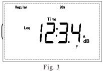
Display the current time HH: MM (hour: minute). When a digit is flashing, you can use the  $\checkmark$  key to modify the time, use the  $\blacklozenge$  key to select the year, month, day, hour and minute to modify. After the modification is confirmed, press the **SET** key to save the current setting and enter the grid number setting. The real-time clock is powered by backup battery. Once set, it can not be changed.
