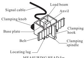
MEASURING HEAD for **BELT TENSION GAUGE**
