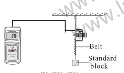
W=W0+W1Here W0 is the weight of standard block, and W1 is the weight of the belt
