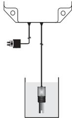
The EC or TDS value automatically compensated for temperature is shown on the primary LCD while the secondary LCD shows the temperature of the sample.
