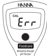
In calibration mode, if the probe is in the correct buffer solution and the "Err" message is displayed, the probe should be cleaned. Soak the probe in cleaning solution for 20 minutes. Rinse with water and hydrate electrode in storage solution for a minimum of 30 minutes before calibrating.
