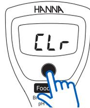
To clear the user calibration and restore the tester to factory default. From calibration mode, press and hold the ON/OFF button, the LCD will show "CLr".
