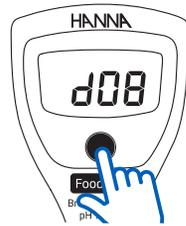
From measurement mode, press and hold the ON/OFF button. The LCD will show "OFF", "CAL" followed by "d08" (default setting, 8 minutes). Release the ON/OFF button. A single press on the ON/OFF button will change the auto-off timer to "d60" (60 minutes). To disable the auto-off feature press the ON/OFF button again, LCD will show "d--". Press and hold to exit.
