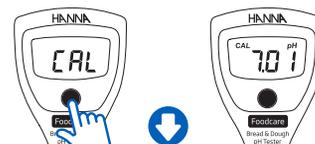
**A** For one or two-point calibration using pH 7.01 buffer solution, follow procedure A.
