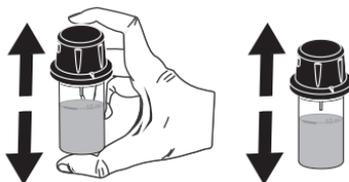
In order to avoid reagent leaking and to obtain more accurate measurements, close the cuvette first with the supplied HDPE plastic stopper
