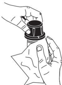
Shaking the cuvette can generate bubbles in the sample, causing higher readings. To obtain accurate measurements, remove such bubbles by swirling or by gently tapping the cuvette.
