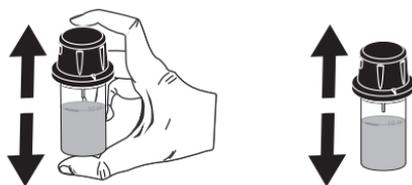
In order to avoid reagent leaking and to obtain more accurate measurements, close the cuvette first with the supplied HDPE plastic stopper
