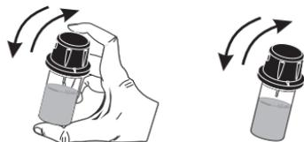
In order to avoid reagent leaking and to obtain more accurate measurements, close the cuvette first with the supplied HDPE plastic stopper
