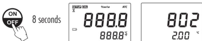
2. While continuing to hold the **ON/OFF** key, press the **ZERO** key. The temperature unit will change from  $^{\circ}\text{C}$  to  $^{\circ}\text{F}$  or vice versa.
