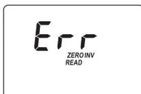
**Inverted Cuvettes:** The sample and the zero cuvette are inverted.
