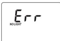
**No Light:** The instrument cannot adjust the light level. Please check that the sample does not contain any debris.
