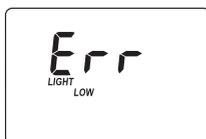
**Light Low:** There is not enough light to perform a measurement. Please check the preparation of the zero cuvette.
