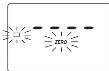
**Battery low:** The battery must be replaced soon.
