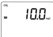
*Note: If the display shows “STD HIGH”, the standard value was too high. If the display shows “STD LOW”, the standard value was too low. Verify that both CAL Check™ Standards HI96753-11 Cuvettes, A and B are free of fingerprints or dirt and that they are inserted correctly.*
