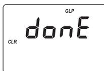
To save battery, the instrument shuts down after 10 minutes of non-use in *measurement mode* and after 1 hour of non-use in calibration mode.
