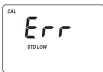
**Standard Low:** The standard reading is less than expected.
