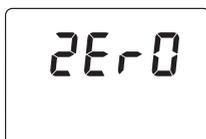
**Zero:** A zero reading was not taken. Follow the instructions of the measurement procedure for zeroing the meter.
