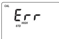
**Standard High:** The standard reading is higher than expected.
