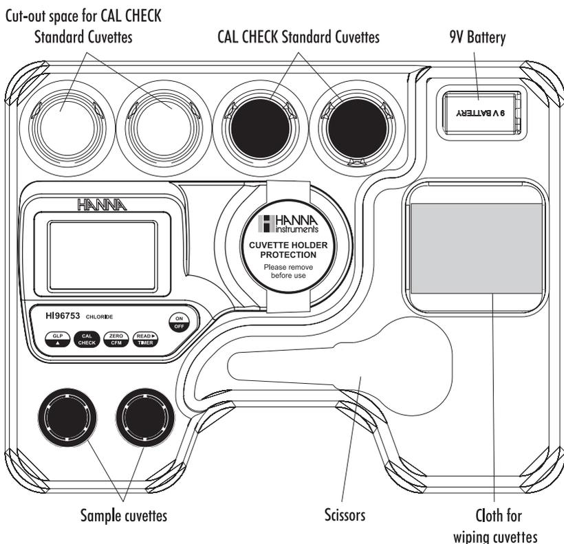
The **HI96753** is an auto diagnostic portable microprocessor meter that benefits from Hanna Instruments' years of experience as a manufacturer of analytical instruments. It has an advanced optical system based on a special Light Emitting Diode (LED) and a narrow band interference filter that allows most accurate and repeatable readings. All instruments are factory calibrated and the electronic and optical design minimizes the need of frequent calibration.
