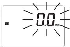
**Under Range:** A blinking “0.0” indicates that the sample absorbs less light than the zero reference. Check the procedure and make sure you use the same cuvette for reference (zero) and measurement.
