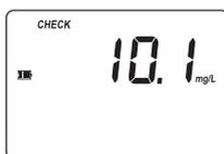
The reading should be within specifications as reported in the **CAL Check™** Standard Certificate. If the value is found out of the specifications, please check that the cuvettes are free of fingerprints, oil or dirt and repeat validation. If results are still found out of specifications, then recalibrate the instrument.
