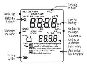
Mode tags light up for indicating the corresponding active mode, and blink for warning the user.
