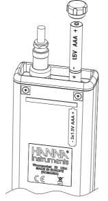
The instrument is provided with the BEPS (Battery Error Prevention System) feature, which automatically turns the instrument off when the batteries level is too low to ensure reliable readings. At start up the display will show "**0 bAtt**" message for a few seconds, then the instrument automatically turns off.
