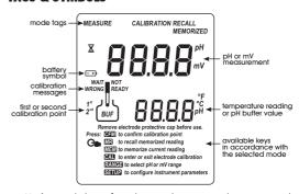
Mode tags light up for indicating the corresponding active mode, and blink for warning the user.
