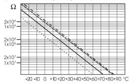
Since the resistance of the pH electrode is in the range of 50-200 Mohms, the current across the membrane is in the pico Ampere range. Large currents can disturb the calibration of the electrode for many hours.
