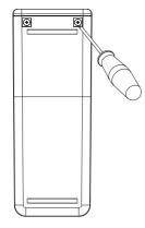
Insert four new 1.2V AAA 1000 mAh NiMH rechargeable batteries in the battery compartment while paying attention to the correct polarity. Make sure that the "Battery type" switch is in NiMH position.
