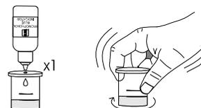
acidic and an acidity test must be carried out (see HI 3820 — Hanna Acidity Test Kit). If the solution is green or blue, then proceed to next step.
