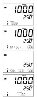
The cell factor in  $\mbox{cm}^{\cdot 1}$  determined from the calibration with the current reading.
