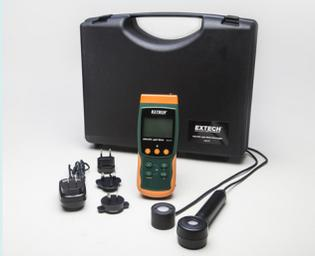
Extech's compact UV Light Meter includes two types of probes: one to measure UVA (long wave 365nm) and the other to measure UVC (short wave 254nm) light sources up to 20mW/cm<sup>2</sup>. The UV800 date/time stamps and stores files onto a 2GB SD card in MS Excel<sup>®</sup> format to make transferring, storing, and analyzing the data on your PC easier. The unit also has a Type K/J thermocouple input to capture temperature readings (probes not included).
