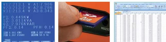
Backlit LCD displays numerical values. The data can be stored in SD memory card (included) and then transferred from meter to PC using Excel<sup>®</sup> software and datalogged readings.
