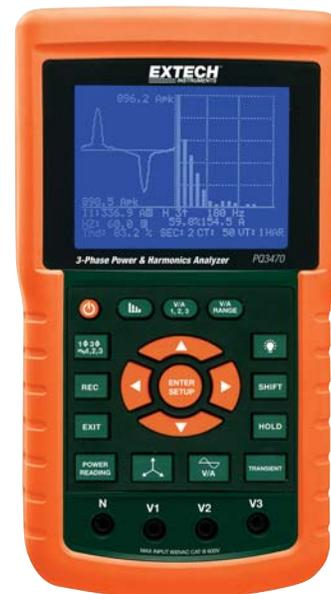
Complete with 4 voltage leads with alligator clips, 8 AA batteries, SD memory card, Universal AC adaptor (100 to 240V), and case. Clamp probes sold separately.
