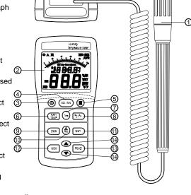
NOTE: Do not immerse the probe in liquid; it is intended for use in air only.
