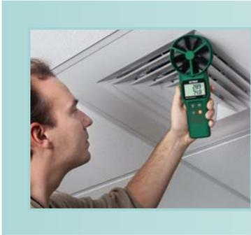
Extech's 4" (10cm) Large Vane Thermo-Anemometer series allows for more precise readings on larger size ducts. Each meter simultaneously displays Airflow or Air Velocity and Temperature. Choose models that also measure Air Volume, Humidity & Carbon Dioxide (CO<sub>2</sub>).
