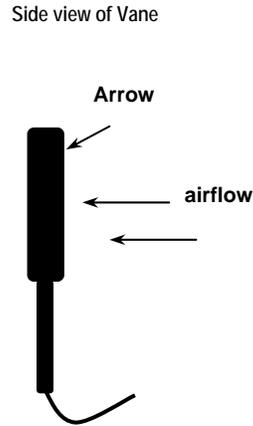
5. Place the sensor in the air stream. Ensure that the air enters the vane as indicated by the arrow sticker placed inside the vane. Refer to the diagram.
