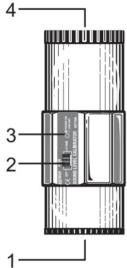
\* To remove the 1/2" adaptor, pull straight down as shown in diagram below.
