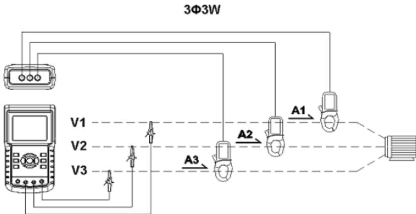
1. Power the instrument ON by pressing the POWER KEY, and then press 1Φ 3Φ KEY to select 3Φ 3W, the selected configuration name will appear on bottom left hand side of the display for screen 2.
