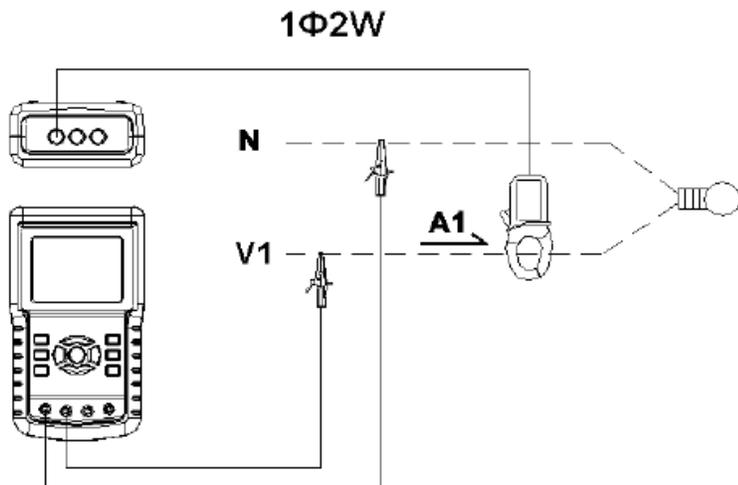
1. Power the instrument ON by pressing the POWER KEY, and then press 1 $\Phi$  3 $\Phi$  KEY to select the 1 $\Phi$  2W system, the selected name of the system will be shown on the bottom left side of the display on screen 2
