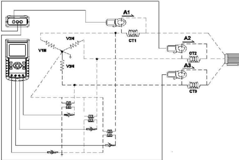
1. Power the instrument ON by pressing the POWER KEY, and then press the 1Φ 3Φ KEY to select the 3Φ 4W system, the selected name of the system will appear on the bottom left hand side of the display for screen 2
