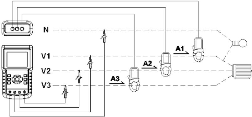
1. Power the instrument ON by pressing the POWER KEY, and then press 1Φ 3Φ KEY to select the 3Φ 4W system, the selected name of the system will appear on the bottom left hand side of the display for screen 2
