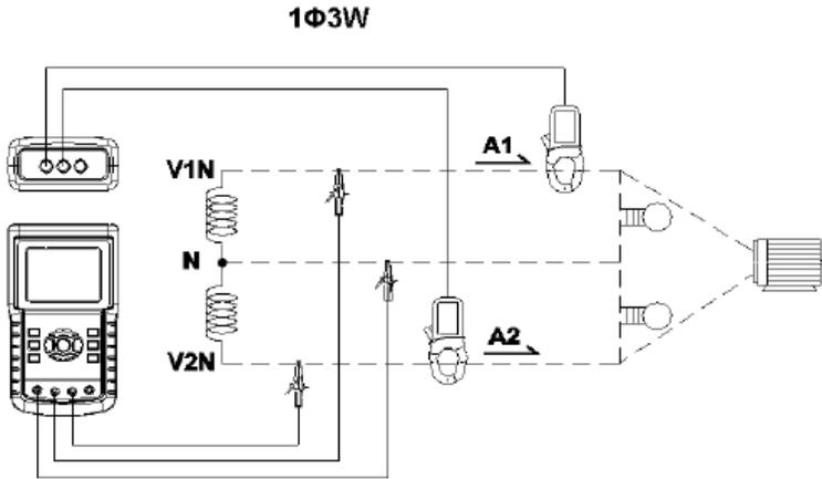
1. Power the instrument ON by pressing POWER KEY, and then press the 1Φ 3Φ KEY to select 1Φ 3W, the selected name of the configuration will appear on bottom left hand side of the display for screen 2.
