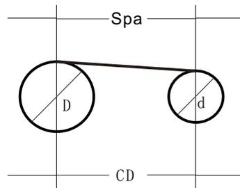
In low tension ranges, a bigger vibration may be generated more easily, which may cause measurement errors. If the tension value cannot be obtained, the belt may be too loose to make a clear frequency signal. For more accurate tension values, try to tighten the belt.
