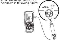
OWind Flow Calculate Formula: Flow =velocity \*(Free Area)
