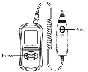
2. After the entire screen displays for 1 second, the default state is acceleration mode, if on the LCD displays the symbol , please promptly replace the battery, as shown in following figure:
