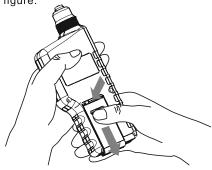
2). Insert the 9V battery into battery compartment, note the battery polarity, and then close the battery door, as shown in the following figure:
